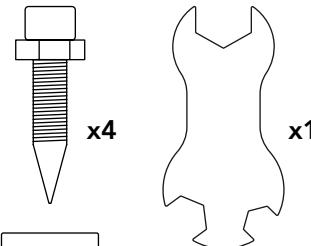
2- Attach the spikes on the bottom plate. The provided nuts enable you to adjust the spikes to assure alignment with your floor. Use the dedicated floor protectors if necessary.
